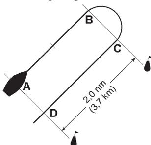
Make a measuring run at a cruising speed, which remains as constant as possible. Check that the trip distance counter is set to zero.
