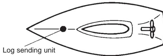
**On sailing boats** the sending unit should always be installed in front of the keel, as close to the longitudinal ship axis as possible. On boats with a long keel the installation should be at the end of the first third of the hull, but not at the widest location of the hull.
