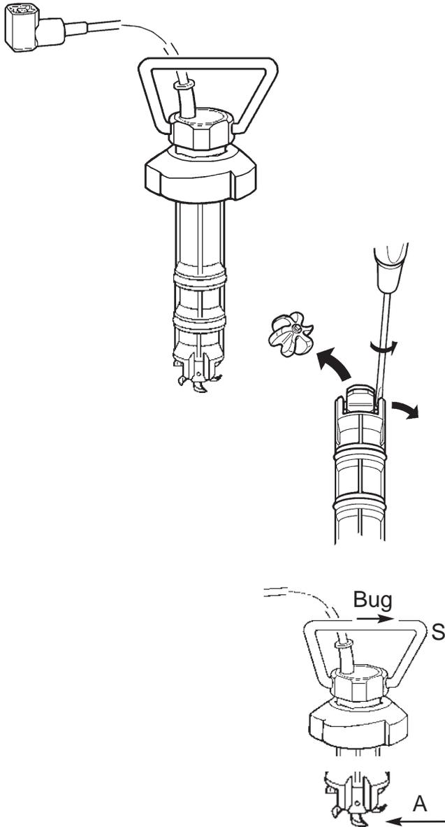
The paddle wheel of the sending unit is rotated by the flow of water. The rotational speed of the paddle wheel is measured without contacts, and transmitted to the indicating instrument.
