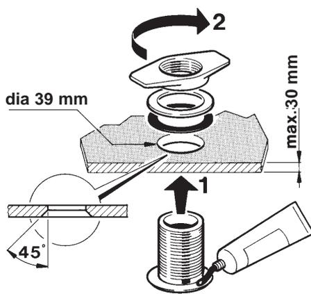
Make a hole 39 mm dia., at a suitable location. The wall thickness can be up to 30 mm. Camber the hole out at 45 degrees for good sealant distribution during the assembly. To install the hull sleeve and the sending unit proceed as follows:
