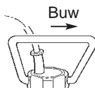
Note the correct direction when inserting the sending unit. The pointed side of the sending unit loop must be directed towards the bow as soon as the sending unit has been inserted.
