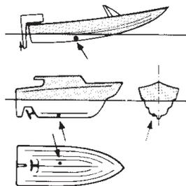
**On powerboats** the sending unit should be installed at about the first third of the hull and never towards the stern in a zone of strong turbulence or up front, where strong disturbances by air induction must be expected. An ideal installation is near the longitudinal axis of the ship and in the zone of the first stringer, directly in front of the engine compartment if possible. At higher speeds this is the only location where a disturbancefree operation can be expected..
